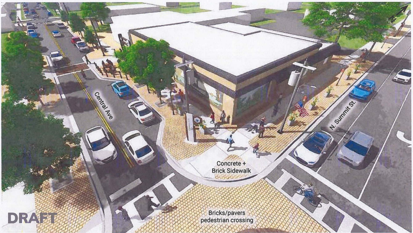
Street Improvement Materials - Central Avenue and Summit Street
